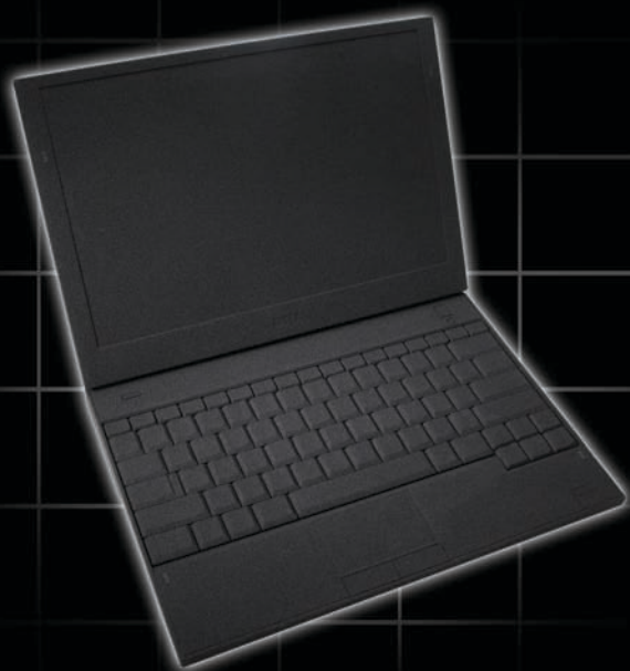
Step 4: Foam models are carved to show the general size and shape of the selected concepts.
