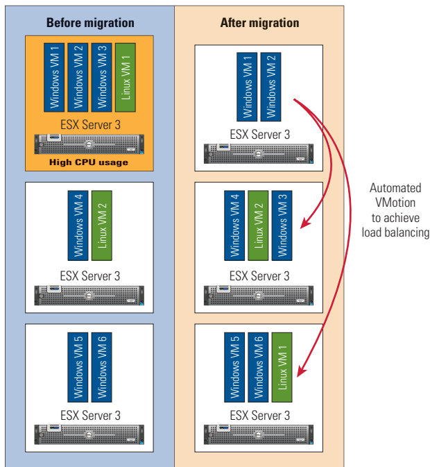
Figure 1. VMware Distributed Resource Scheduler and VMotion migrating virtual machines to a new location to achieve load balancing
