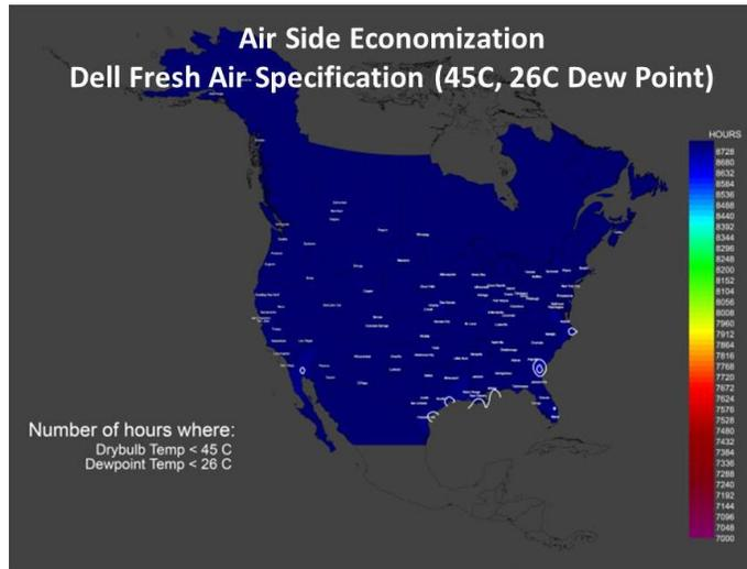
Note on Figure 5: With the Dell fresh air capable IT equipment specifications of 45°C and a 26°C maximum dew point, the dark blue region corresponding to economization for 100% of the hours in a year (chiller-less fresh air cooling) envelopes almost the entire North American continent.
