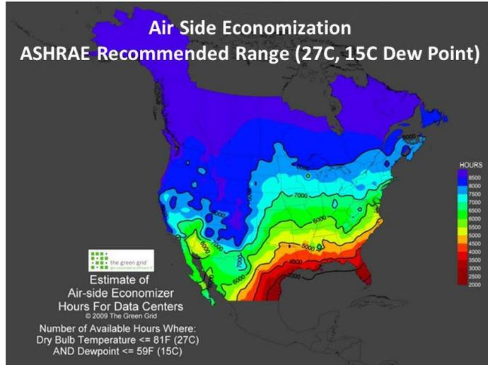
Note on Figure 4: The geography suitable for a chiller-less fresh air cooled data center (economization for 100% of the hours in a year) corresponds to the dark blue region in Alaska and northernmost Canada. The remaining regions below the dark blue region would all require a chiller plant, air conditioning system, or other supplemental cooling capability.
