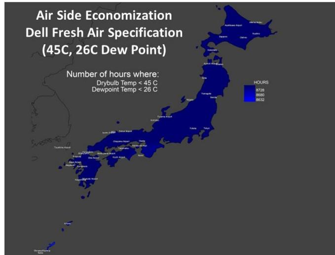
Note on Figure 7: With Dell fresh air rated IT equipment, a chiller-less data center could be built almost anywhere in Japan. The darkest shade of blue corresponds to economization for 100% of the hours in a year.
