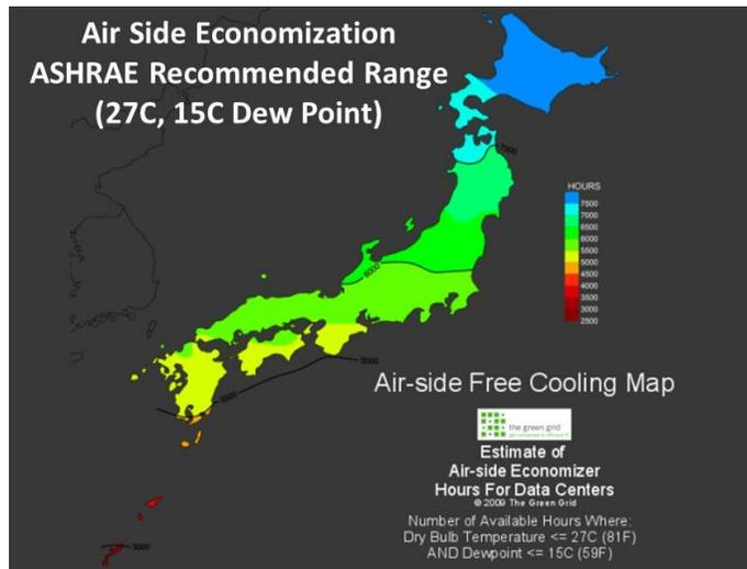
Note on Figure 6: Under the assumed conditions of 27°C maximum dry bulb temperature and a maximum dew point of 15°C, none of the islands of Japan are suitable for chiller-less fresh air cooling. Any data center built under these temperature assumptions would have to bear the capital cost of installing a chiller, air conditioner or some kind of cooling plant.
