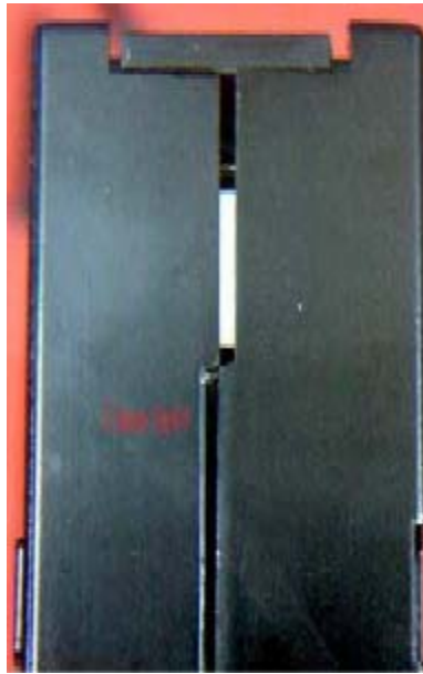
Figure 17- Split seam on LTO tape
