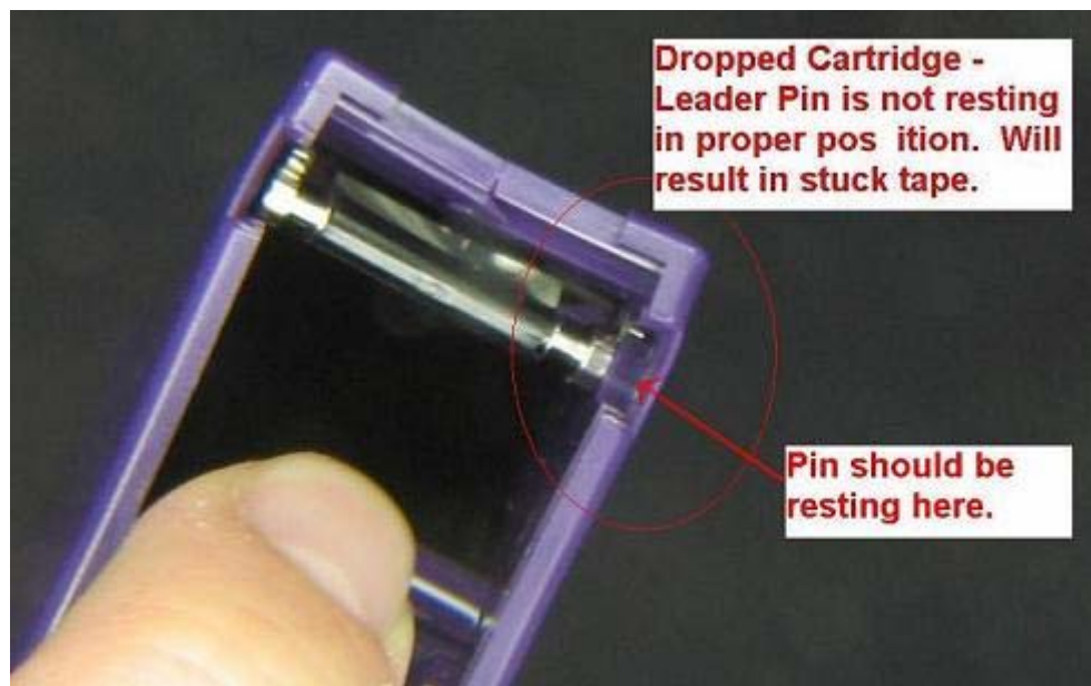
Figure 16 Media Inspection 1- bad tape
