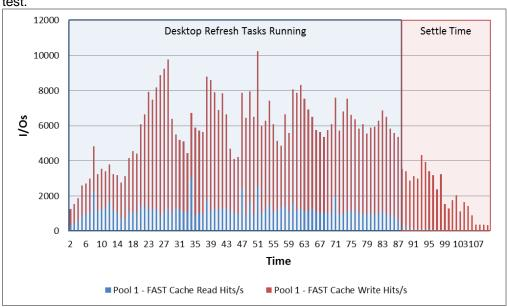
At peak load, FAST Cache serviced over 10,000 IOPS from the linked clone datastores, which is the equivalent of 50 FC disks serving 200 IOPS each.
