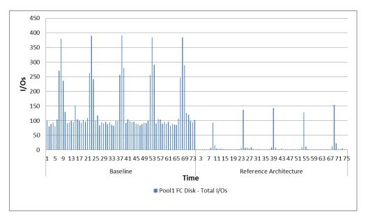
FAST Cache reduced the peak load on the disks from 391 IOPS to 154 IOPS, which is more than two times decrease in the I/Os required to be serviced from the pool disks.
