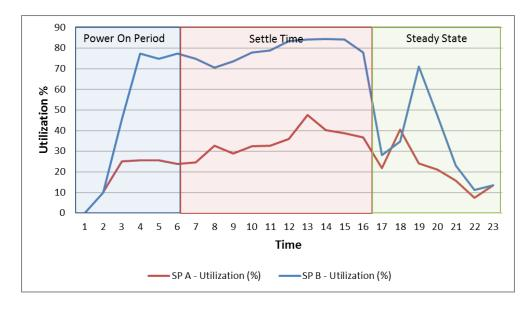
The replica traffic caused high SP utilization during the peak load of the test. For a better distribution of the load, place the replica images on separate storage processors.
