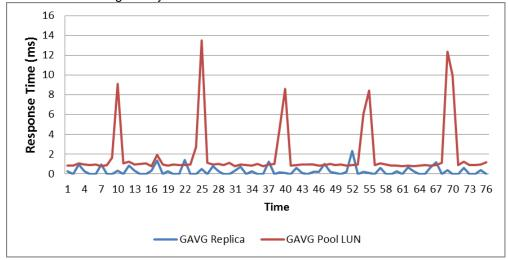
GAVG for both the EFDs, replica storage and linked clone storage on the Pool1\_x datastores were well below 20 ms for the entire test.
