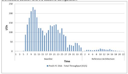
FAST Cache reduced the peak load on the disks from 232 IOPS to 13 IOPS, nearly an 18 times decrease in the I/O required to be serviced from the pool disks. Additionally, the time to boot all desktops to steady state was decreased from 21 minutes to 13 minutes in the reference architecture solution.
