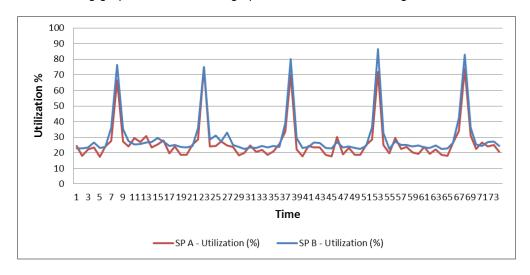
The replicas were owned by SP B, which caused all reads to be handled by SP B. This resulted in throughput and utilization of SP B to be higher than those of SP A. The patch install for each desktop collection caused high CPU utilization briefly during peak load. However, the headroom was still available.
