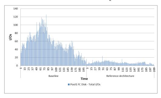
FAST Cache reduced the peak load on the disks from 125 IOPS in the baseline configuration to 23 IOPS in the reference architecture solution, which was a decrease of more than five times in the I/Os to be serviced from the pool disks.
