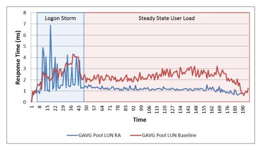
GAVG for both the EFD replica storage and linked clone storage on the Pool1\_x datastores were well below 10 ms during this test.
