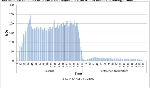
FAST Cache reduced peak load on the disks from 245 IOPS in the baseline configuration to 16 IOPS in the reference architecture solution — which is more than 15 times reduction in the I/O required to be serviced from the pool disks.
