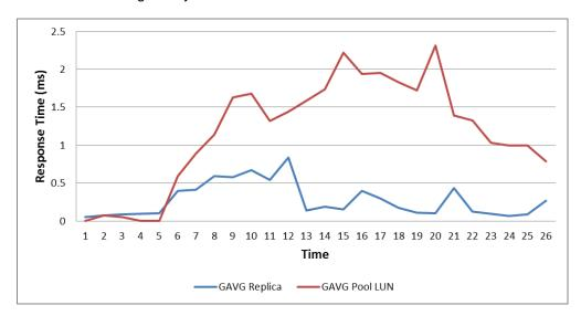
GAVG for the EFD replica storage and the linked clone storage on the Pool1\_x datastores was less than 2.5 ms. This indicates excellent performance under this load.
