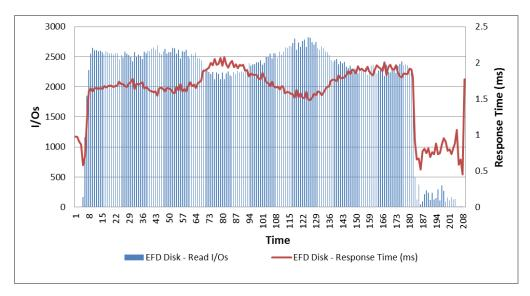
Each EFD was servicing over 2,700 IOPS at peak load, but the response time remained below 2 ms. This indicates that the disks were not driven to saturation.
