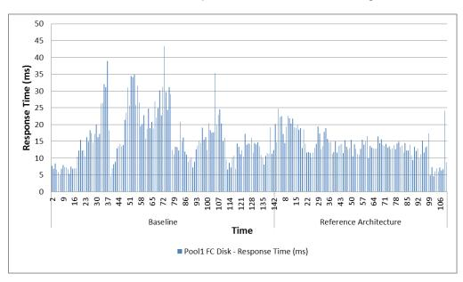
The peak disk response time was reduced by approximately 50 percent in the reference architecture solution when compared to the baseline configuration.
