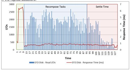
The copy of the new replica image caused a heavy sequential write workload on the EFDs, thus causing a small spike in the response time, up to a peak of 6.5 ms for the EFDs.
