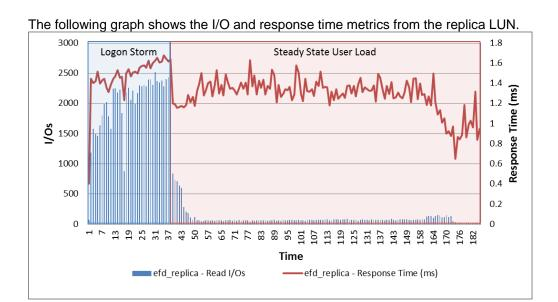
The replica LUN serviced nearly 2,500 IOPS during peak load with a maximum response time of less than 2 ms, which indicates that the LUN was not driven to saturation.
