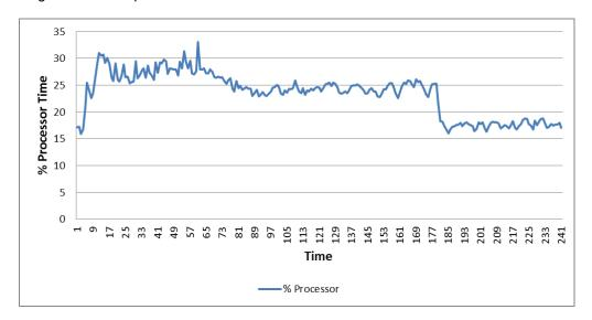
The CPU load on the ESX server was well within the acceptable limits during this test.
