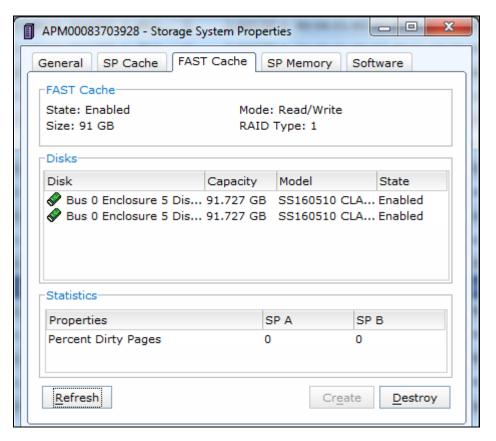
FAST Cache is not enabled for the replica storage in this solution. The replica images are serviced from the EFDs. Enabling FAST Cache for these LUNs causes additional overhead without added performance.
