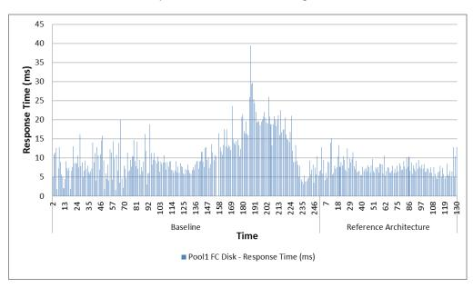
The disk response time stayed well below 15 ms for the duration of the test in the reference architecture when compared to a peak of 39 ms in the baseline configuration.
