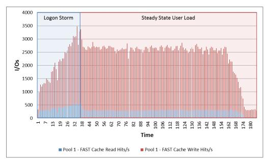
FAST Cache serviced over 3,500 IOPS at peak load from the linked clone datastores, which is the equivalent of 18 FC disks serving 200 IOPS each.
