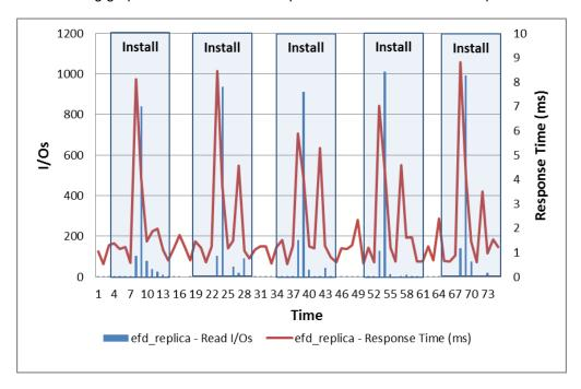
The replica LUN serviced over 1,000 IOPS during peak load with a maximum response time below 10 ms, which indicates that the LUN was not driven to saturation.
