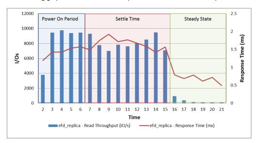
The replica LUN serviced nearly 10,000 IOPS during peak load with a maximum response time of less than 2 ms, which indicates that the LUN was not driven to saturation.
