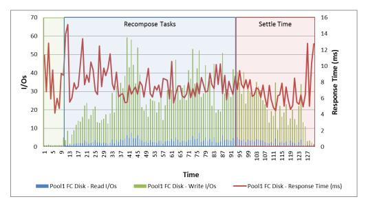
Each drive was servicing fewer than 60 IOPS at peak load and the response time for the drives remained below 10 ms. This indicates that the disks were not driven to saturation.
