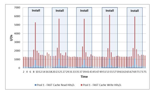
The FAST Cache serviced over 6,200 IOPS at the peak load from the linked clone datastores, which is the equivalent to 31 FC disks servicing 200 IOPS each.
