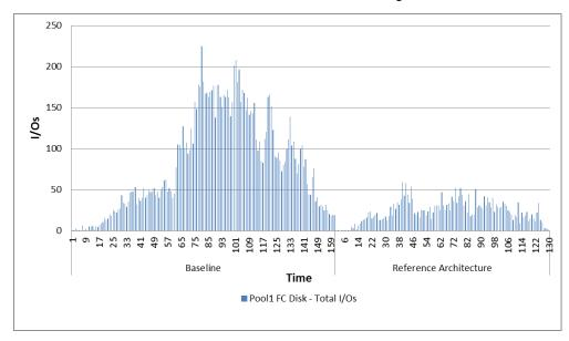
FAST Cache reduced the peak load on the disks from 224 IOPS in the baseline configuration to 59 IOPS in the reference architecture solution, which was a decrease of more than three times in the number of I/Os to be serviced from the pool disks.
