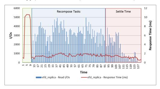
The replica LUN serviced nearly 5,000 IOPS during peak load with a maximum response time of less than 2 ms. This indicates that the LUN was not driven to saturation during the actual deployment of new desktops.
