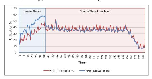
The storage processor utilization peaks at 58 percent during the logon storm. The steady state performance was stable with a utilization of 40 percent on both storage processors.
