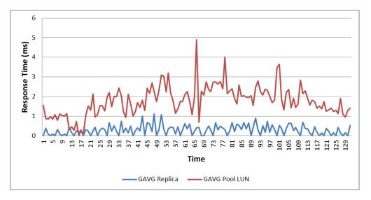
GAVG for both the EFD replica storage and the linked clone storage on the Pool1\_x datastores was below 5 ms. This indicates a very good performance under this load.
