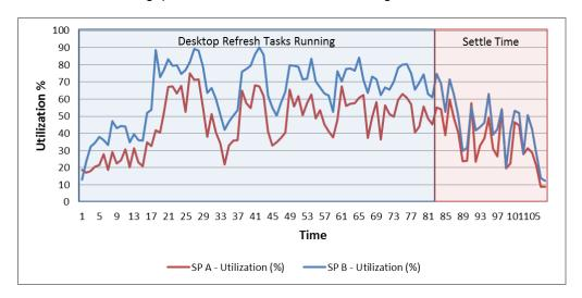
The refresh operation caused high CPU utilization during peak load, but headroom was still available.
