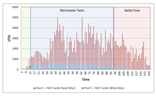
At peak load, FAST Cache serviced over 5,000 IOPS from the linked clone datastores, which is the equivalent of 25 FC disks serving 200 IOPS each.
