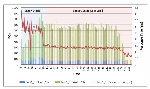
During peak load, the LUN response time never moved above 4 ms while the datastore serviced over 900 IOPS during peak load.
