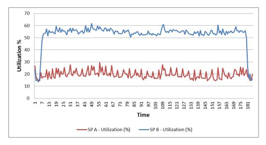
SP B owned all replica images, thus causing its utilization to be high compared to that of SP A, but there was still headroom available on the storage processor. Performance can be improved by splitting the replicas between both storage processors.
