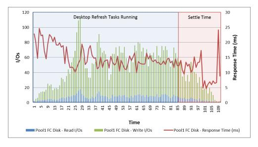
During the peak I/O load, the disk response time was consistently below 20 ms. This indicates that the disk was not saturated. At the beginning and at the end of the test, I/Os serviced by the individual drives in the pool were extremely low. This was because all I/O requests were serviced by FAST Cache.
