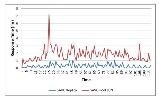
GAVG for the EFD replica storage and the linked clone storage on the Pool1\_x datastores was well below 10 ms, which indicates a very good performance under this load.
