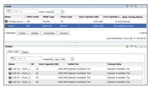
For each LUN in the storage pool, the tiering policy is set to **Highest Available Tier** to ensure that all frequently accessed desktop data remains on the FC disks. As data ages and is used infrequently, it is moved to the SATA drives in the pool.
