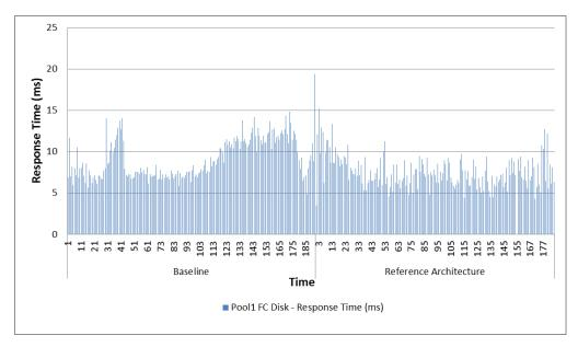
The disk response time stayed below 15 ms for the duration of the test on the reference architecture solution.
