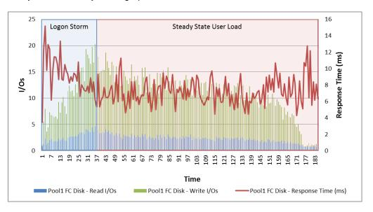
I/Os serviced by the individual drives in the pool were extremely low because nearly all I/O requests were serviced by FAST Cache. The response time appeared relatively high given the disk load. But, this was misleading.
