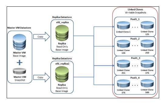
In this configuration, the operating system reads from the common read-only replica image and writes to the linked clone. Any unique data created by the virtual desktop is also stored in the linked clone. A logical representation of this relationship is shown in the following diagram:
