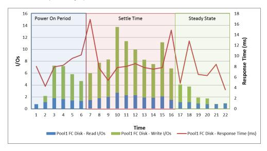
The number of I/Os serviced by the individual drives in the pool was extremely low. This was because nearly all the I/O requests were serviced by FAST Cache. The disk response time appeared relatively high against the load, but this was misleading.
