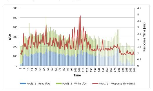
During peak load, the LUN response time remained within 4 ms and the datastore serviced over 500 IOPS.
