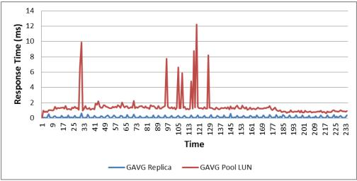
GAVG for both the EFD replica storage and the linked clone storage on the Pool1\_x datastores was well below 10 ms for the majority of the test, with a single spike to 10 ms.
