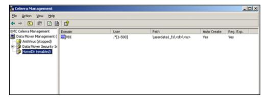
For any user account that ends with a suffix between 1 and 500, the sample configuration shown in the following figure automatically creates a user home directory on the \userdata1\_fs file system in the format \userdata1\_fs\<domain>\<user> and maps the H:\ drive to this path. Each user has exclusive rights to the folder.
