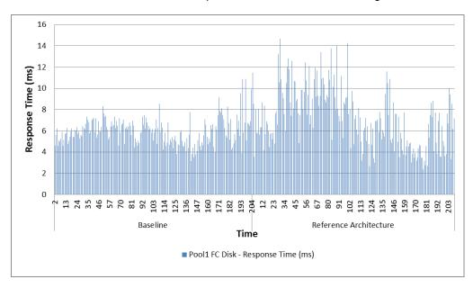
The disk response time stayed below 15 ms for the duration of the test in the reference architecture.
