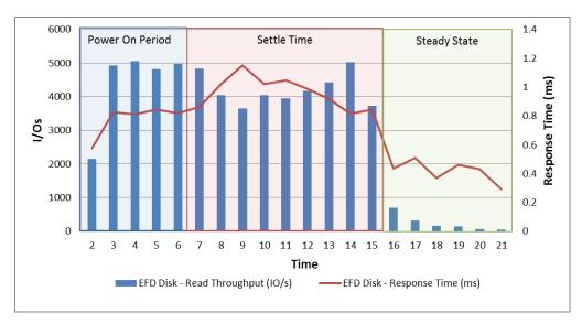
Each EFD serviced 5,000 IOPS at peak load, but the response time for the EFDs remained below 1.2 ms, which indicates that the disks were not driven to saturation.
