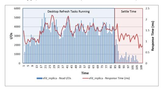
The replica LUN serviced nearly 5,500 IOPS during peak load with a maximum response time of less than 2.2 ms, which indicates that the LUN was not driven to saturation.
