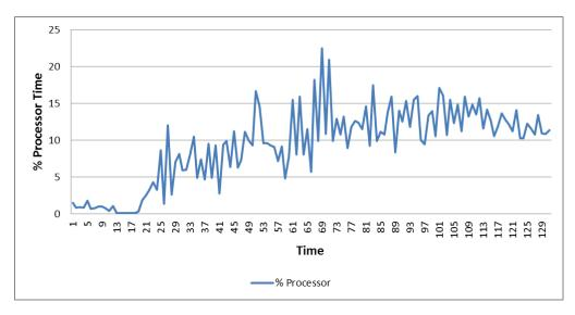
The CPU load on the ESX server was well within acceptable limits during this test.
