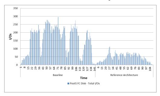
FAST Cache reduced the peak load on the disks from 295 IOPS in the baseline configuration to 109 IOPS in the reference architecture solution, which is a decrease of nearly three times in the I/Os required to be serviced from the pool disks.
