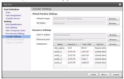
12. In the **Select Datastores** page, select **Use different datastore for View Composer replica disks** and select the datastores for replica and linked clone images, as shown in the following figure.
