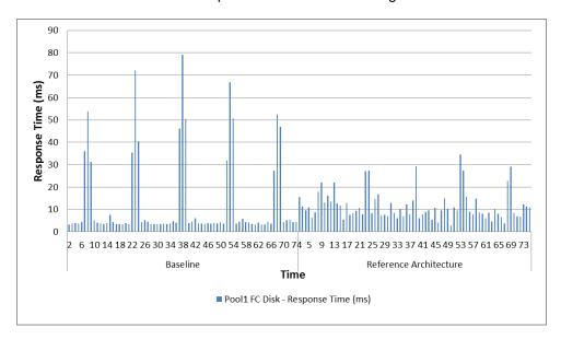
Disk response is significantly reduced during the patch test with FAST Cache. The response time remained below 34 ms for the duration of the test for this reference architecture, and for the baseline configuration, it peaked over 78 ms.
