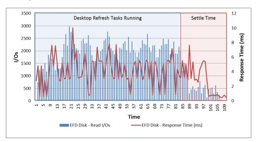
Each EFD was servicing nearly 3,000 IOPS at peak load, but the response time for the EFDs remained below 10 ms, which indicates that the disks were not driven to saturation.
