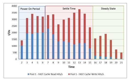
At peak load, FAST Cache serviced over 3,700 IOPS from the linked clone datastores, which is the equivalent of 18 FC disks serving 200 IOPS each.
