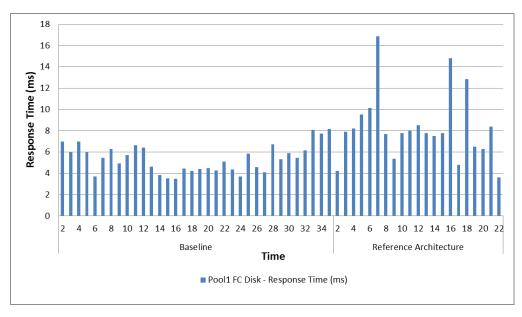
The number of I/Os serviced by the individual drives in the pool was extremely low because nearly all the I/O requests were serviced by FAST Cache. The requests that were serviced by the drives tend to have a very poor locality of reference, which
