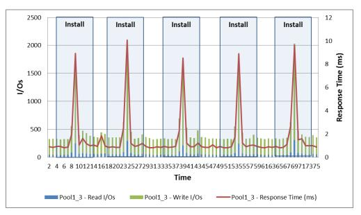
During the peak load, the LUN response time did not move above 10.5 ms when the datastore serviced over 2,000 IOPS during the peak load.
