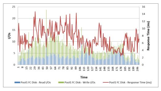
I/Os serviced by the individual drives in the pool were extremely low because nearly all I/O requests were serviced by FAST Cache. The response time appeared relatively high given the disk load, but this is misleading.
