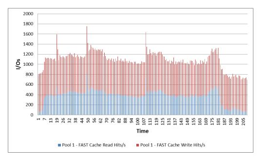
At peak load, the FAST Cache serviced over 1,700 IOPS from the linked clone datastores, which is the equivalent of eight FC disks serving 200 IOPS each. The majority of the read operations are serviced from the replica during this test.
