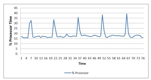
The ESX server CPU load was well within the acceptable limits during the duration of this test.
