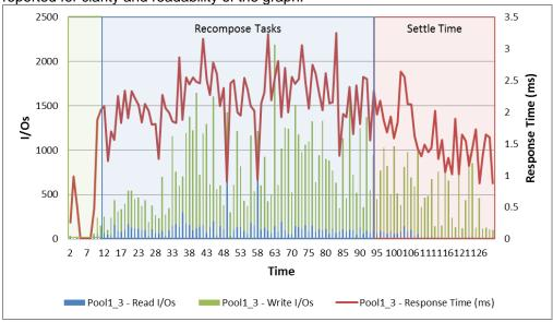
During peak load, the LUN response time remained within 3.5 ms and the datastore serviced over 2,200 IOPS.
