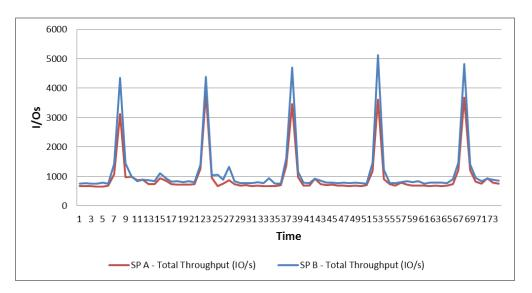
The replicas were owned by SP B, which caused all reads to be handled by SP B. This resulted in throughput and utilization of SP B to be higher than those of SP A.
