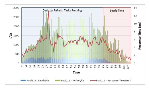
During peak load, the datastore serviced over 2,800 IOPS and the LUN response time remained within 13 ms.
