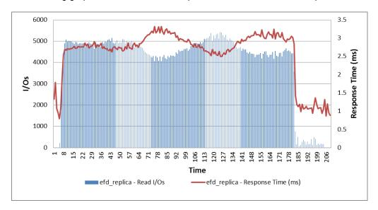
The replica LUN serviced nearly 5,300 IOPS during peak load with a maximum response time of less than 3.25 ms.
