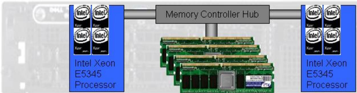
Figure 1 Simplified processor and memory architecture in Dell PowerEdge 2950.
