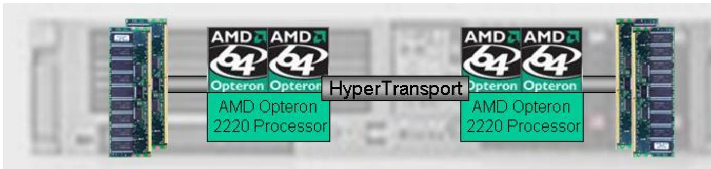
Figure 2 Simplified processor and memory architecture in HP Proliant DL385 G2.
