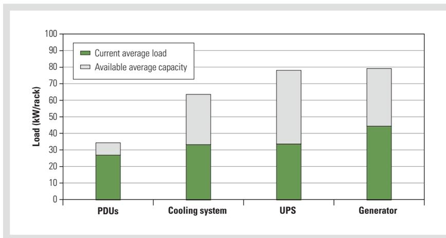
**Figure 3.** Example comparison of average load density with available capacity
