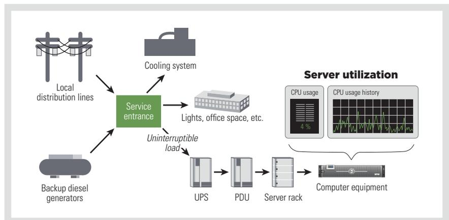
**Figure 2.** Facilities and IT components that contribute to energy usage
