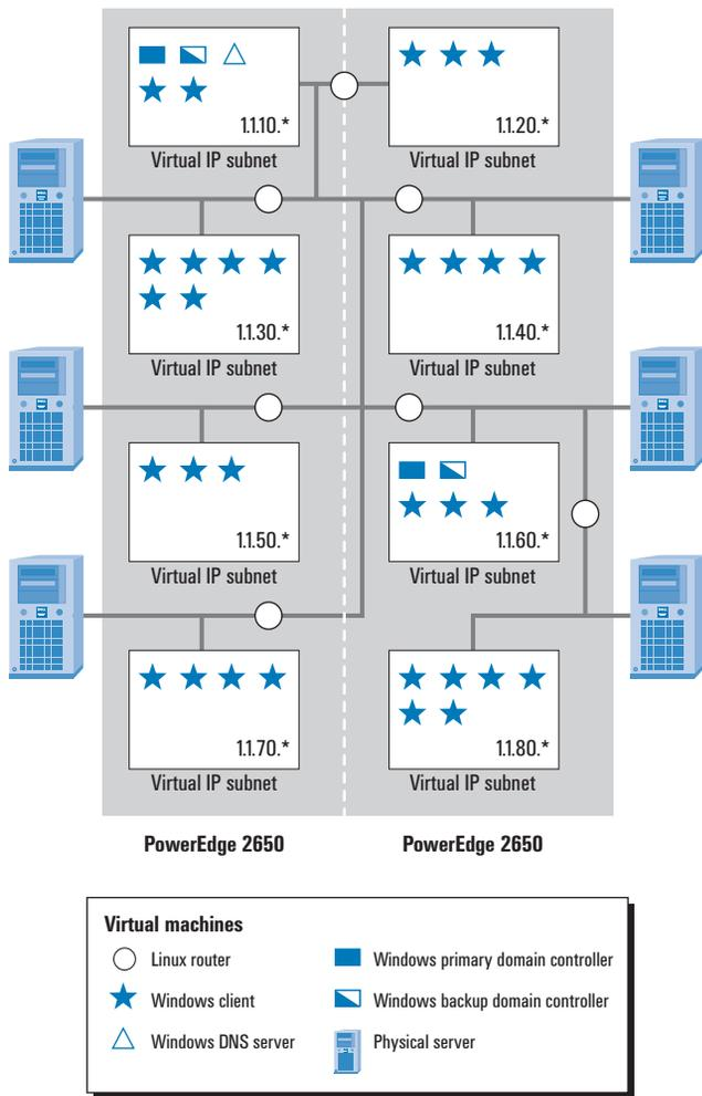
Figure 2. Virtualized network test environment for Active Directory client
