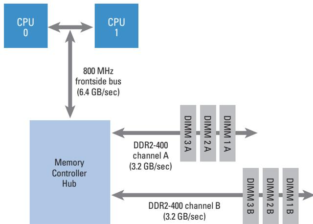
Figure 1. Memory subsystem on PowerEdge 1850, PowerEdge 2800, and PowerEdge 2850 servers
