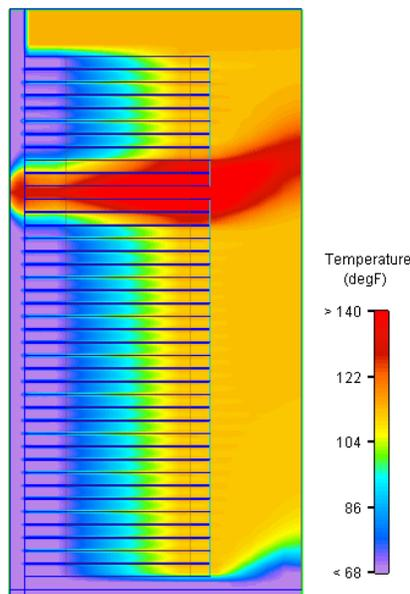
**Figure 2.** CFD Model (Rack Side View): Effect of Not Using a Blanking Panel
