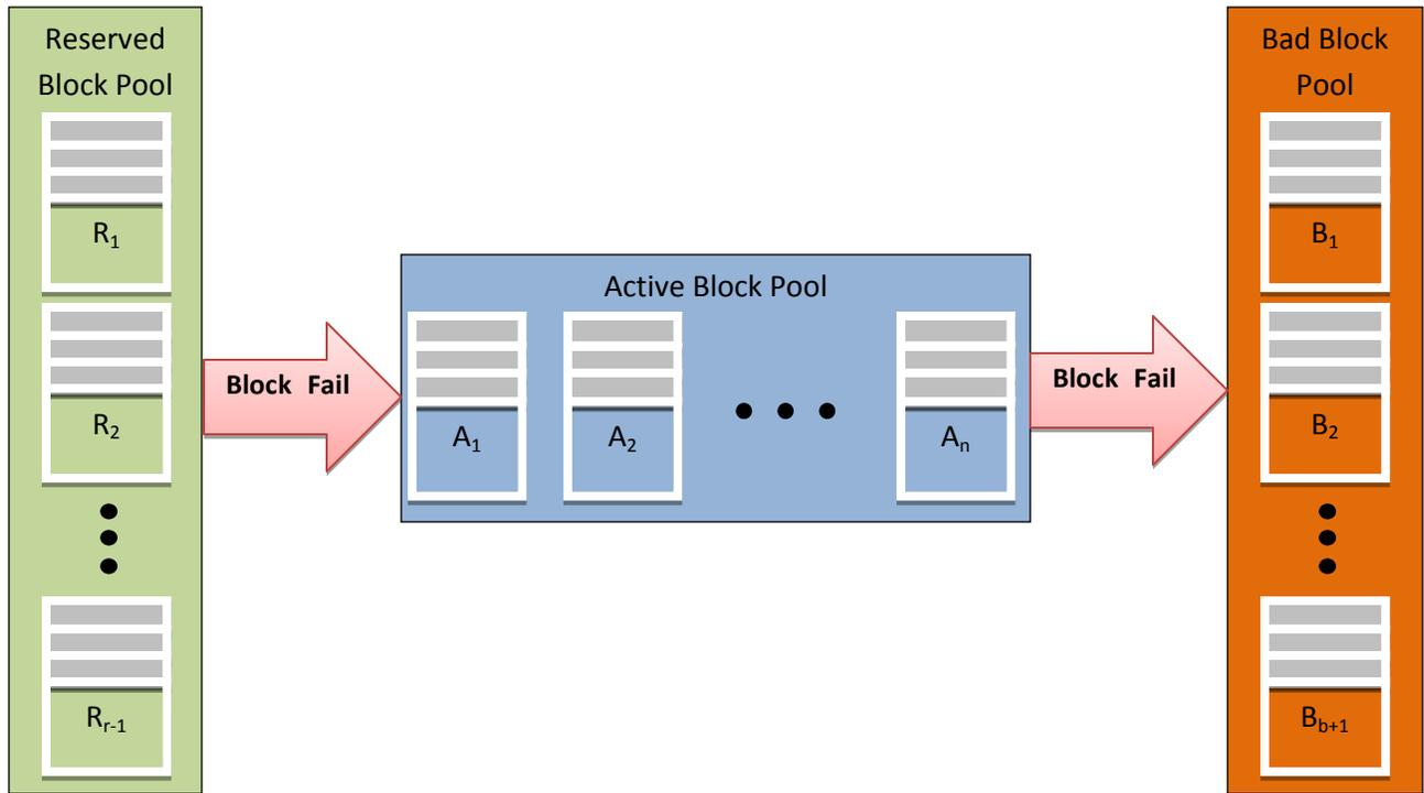
Figure2: Active, reserved, and bad block pool illustration after a block failure
