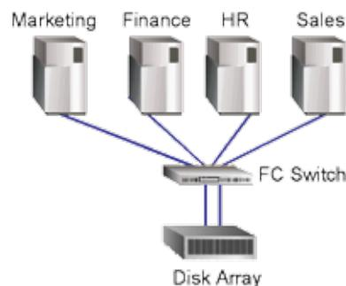
**Figure 6: FC SAN Non-redundant Switch Configuration**
