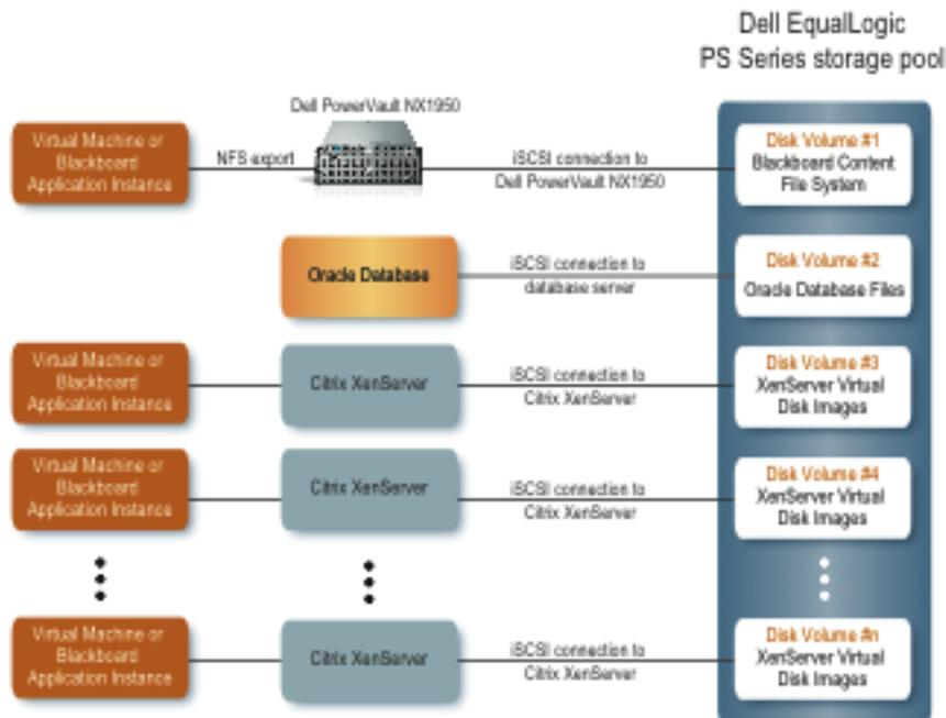
Figure 2: Flexible storage architecture based on Citrix XenServer
