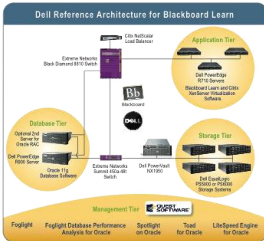
Figure 1: Logical Diagram of Dell Reference Architecture for Blackboard Learn
